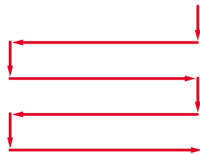
Cutting direction changes along the cutting path
